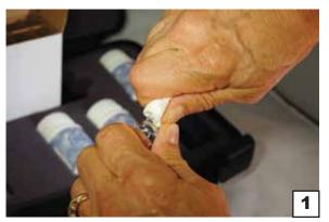
**1.** Turn on the eXact® Micro 10 (M10) Photometer, rinse CELL three times with clean water, and empty CELL.
