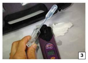
**3.** Take the supplied plastic pipette, squeeze bulb with finger and thumb to expel air, and dip pipette tip to the bottom of ampoule. Release the squeezed bulb to slowly fill the pipette (see *Image 3*). Transfer liquid in the pipette to photometer CELL (see *Image 4*).
